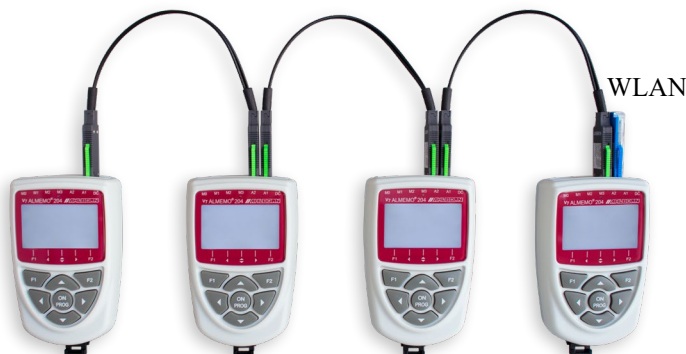
Wired network, up to 99 devices, up to 50 m cable length
