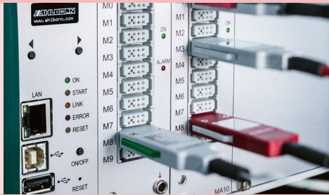
Ports for ALMEMO® sensors and for networking (OLED status display)
